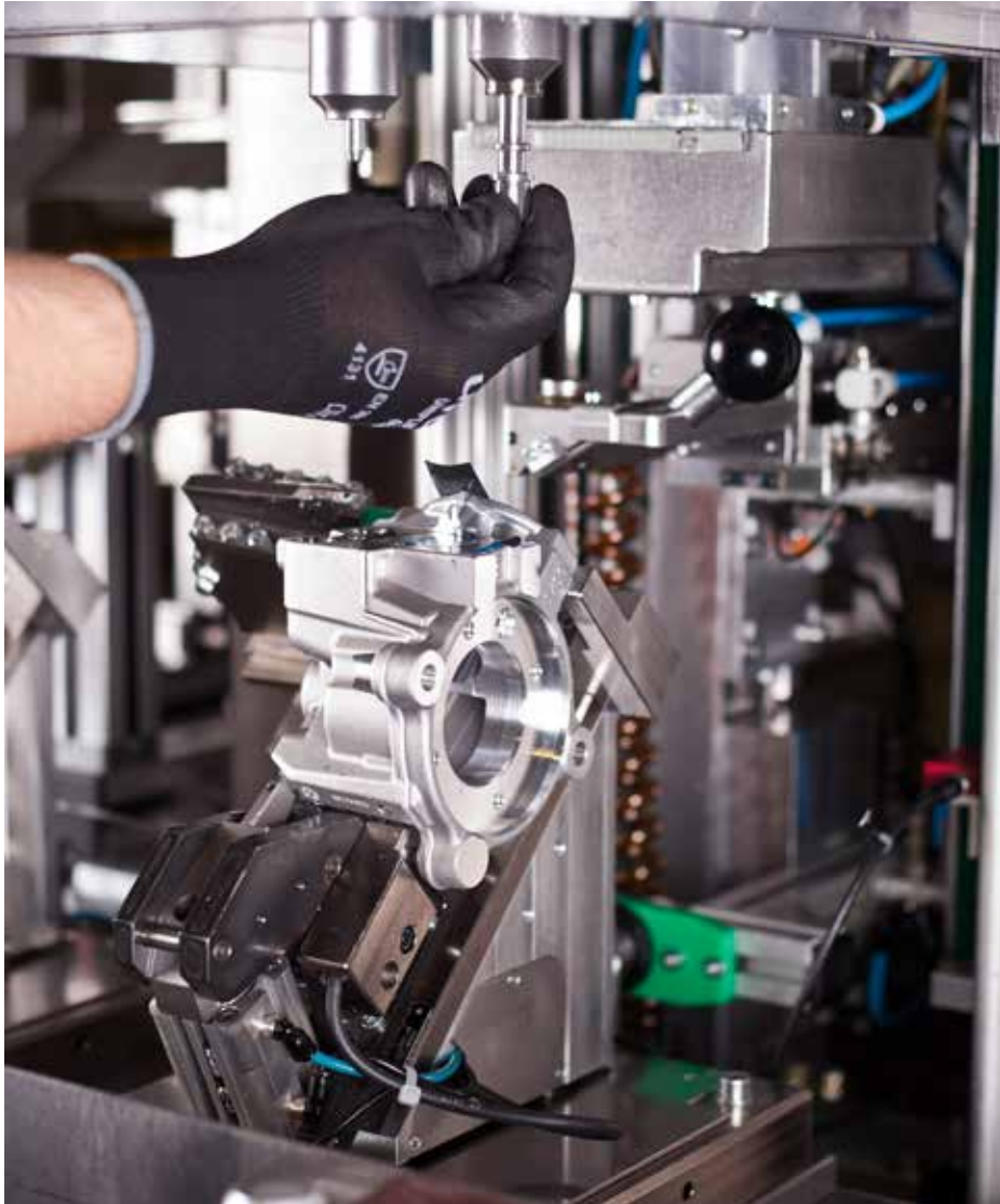
Figure 33: Ergonomic design of a part feeding system
