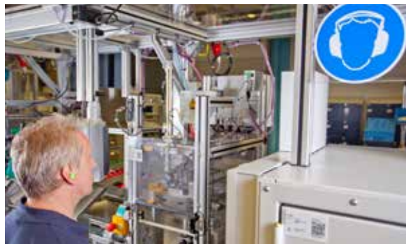
Figure 7: Associate wearing ear protection as per the illustration on the right
