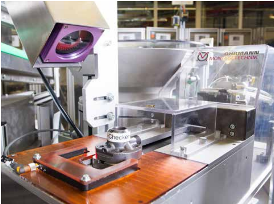
Figure 15: Function test of an automatic camera system using a “check the checker” part
