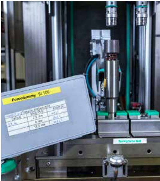
Figure 16 (left) and Figure 17 (right): Application of "check the checker" through inspection of the insertion force sensor using a spring force dummy
