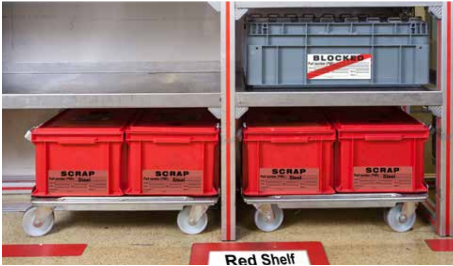
Figure 30: Red shelf with scrap and blocked goods
