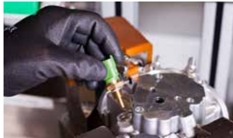
Figure 35 (left): Poka Yoke solution for retaining the correct housing variants Figure 36 (right): Customer-specific color coding of a connector
