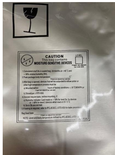
Figure 6: Example of ESD protective MBB bag.
