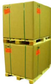
Figure 11: Dynamic stacking factor at least = 2 (1+1).
