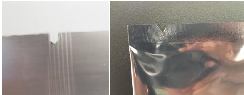
Figure 4: “V” cut shape for opening the MBB bag.
