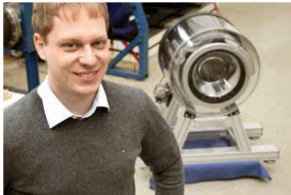
10:38 Using a transparent washing machine, Tobias Morgenthal and his students look at the way textiles move in the drum.
