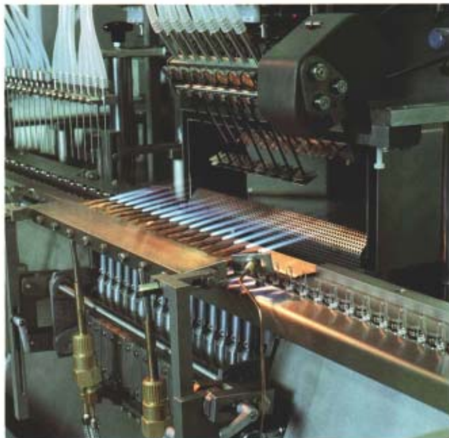
High-quality packaging machinery from our Crailsheim plant: Filling and sealing machine for ampules.
