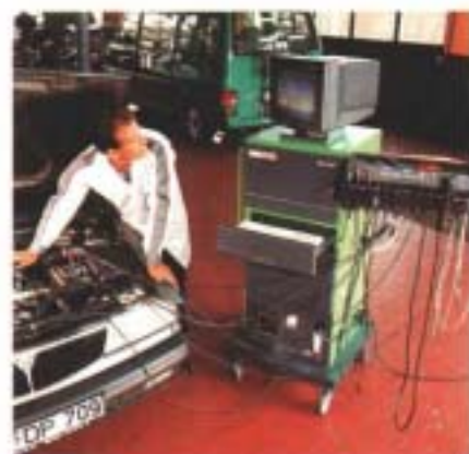
Test equipment for automotive workshops: Efficient analyzers with all functions for a comprehensive engine test on gasoline and diesel engines
