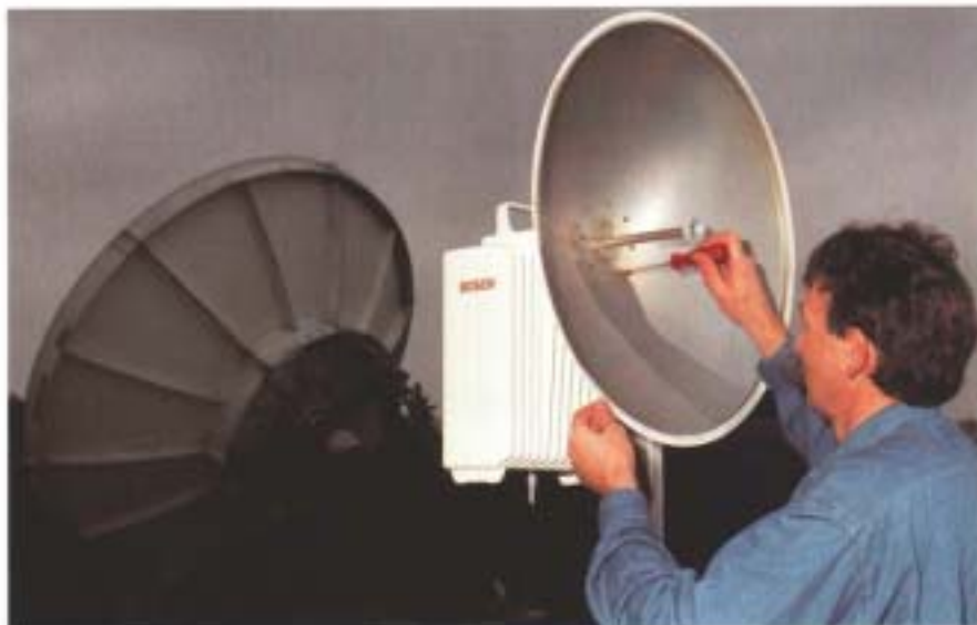
A new cost-effective broadband microwave radio system for short-haul transmission of up to 30 kilometers. It is especially compact and completely compatible with networks based on Synchronous Digital Hierarchy (SDH) technology.
