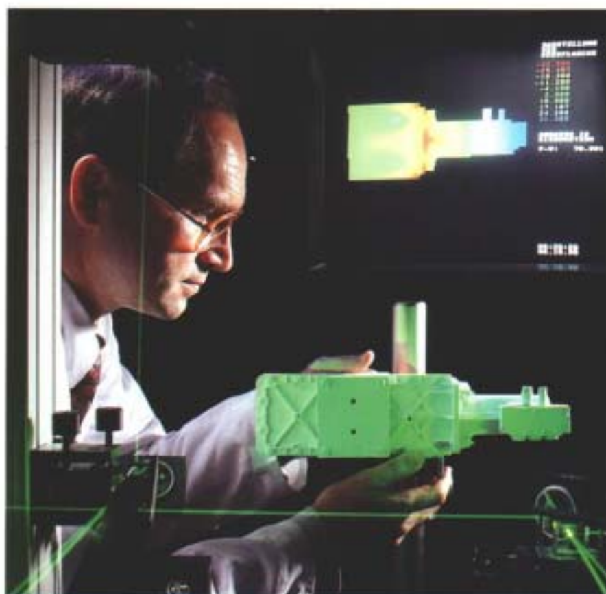
Analysis of the material properties of components. The deformation caused by the laser beam is recorded and evaluated with the aid of TV holography.
