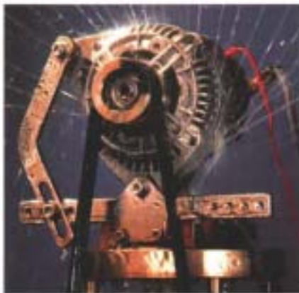
Automotive equipment must withstand the severest stresses. Here our compact alternator is subjected to a splash-water test.
